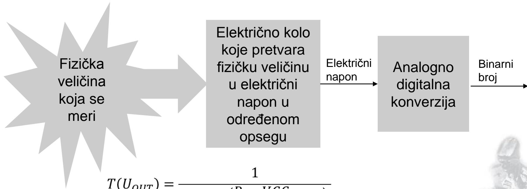
$$T(U_{OUT}) = \frac{1}{\frac{1}{T_0} + \frac{\ln\left(\frac{R_0 * VCC}{U_{OUT}} - R_0\right)}{\beta}}$$
